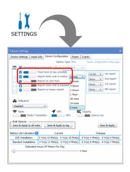
Switch on 'Motion Detection', in device settings (screwdriver & spanner icon on device tile), if you are leaving equipment on site for any period of time. You could set up a motion alert, by switching 'Report when unit in motion' to on.
