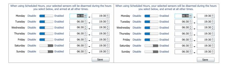
With units running Firmware version 2.20 or later, there is an additional configuration feature available. The option to be able to see a schedule against motion, light, tilt and heavy impact detection.
